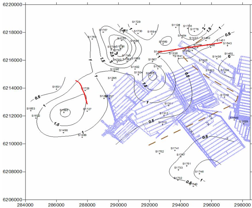
Fig. 4 - Cumulative thickness of gas intervals in the Scarborough Sandstone
