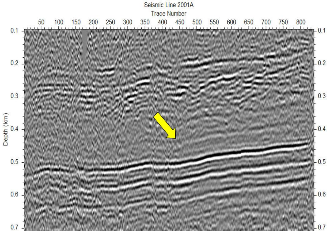
**Fig. 7 - Disrupted seismic reflectors in the Scarborough Sandstone**
