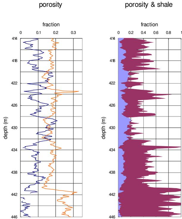
Fig. 3 - Porosity cross-overs in the Scarborough Sandstone
