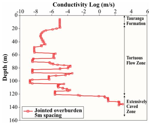
Fig 6: Vertical conductivity profile for N51 panel model.
