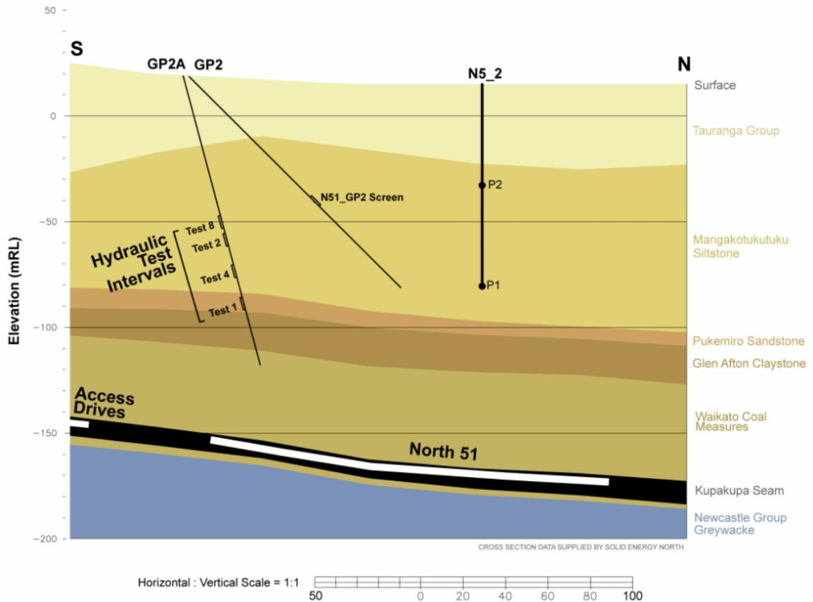
Fig. 2: General stratigraphic section and test borehole locations.
