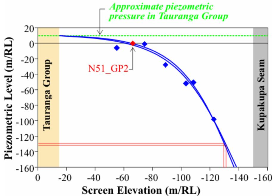
NOTE: Free form best fit curves fitted to data points indicate piezometric elevation coincides with stratigraphic elevation at between -129m/RL and -131m/RL
