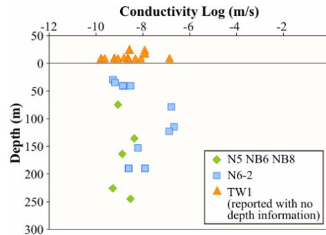
Fig 4: Field packer test data used as background information for insitu conductivity.
