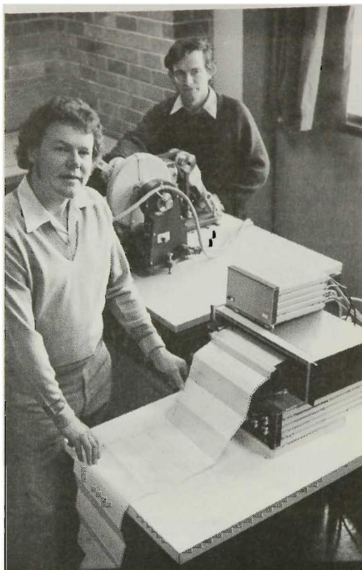
DEPARTMENT of Geology staff, Dr. Bryan Chenhall (left) and Dr. Brian Jones, with the \$39,970 X-Ray Diffractometer which has been installed in Room G11 in the A.C.S. Building. The diffractometer will be used by a number of departments, including Geography, Geology, Metallurgy and Physics.
