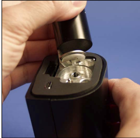
Fig. 3 - Installing a sample filter in the mass sensor
