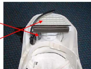
Fig. 20 - Photographs of air stream helmet and the filters used
