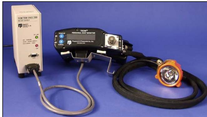
Fig. 2 - PDM installed on charging/communication module
