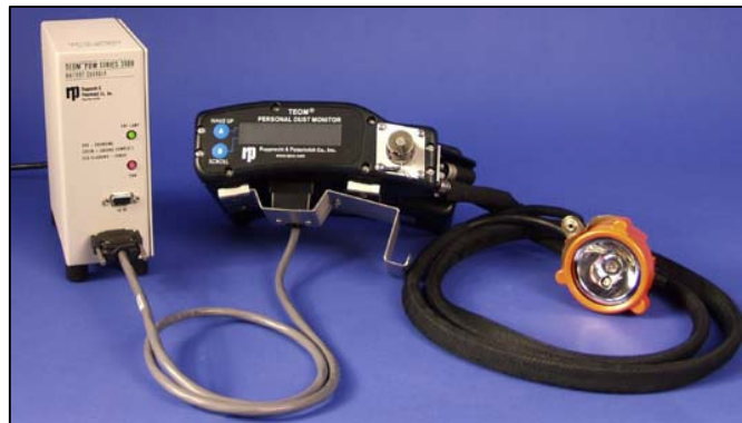
Fig. 2 - PDM installed on charging/communication module
