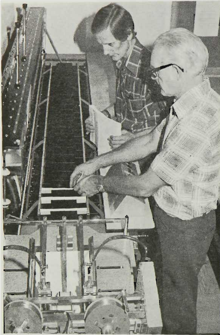
STACKING paper in the bins of the Ordinamatic 24-Station Collator in the University Printery are Lithographic Operator, Mr. Col Hart (foreground), and Office Manager, Mr. Harry Alla.
