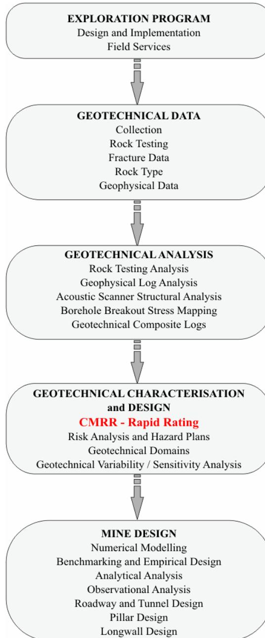
**Fig 4: Geotechnical assessment and design with CMRR.**
