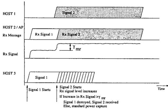
Fig. 3. Operation of the Message Retraining model
