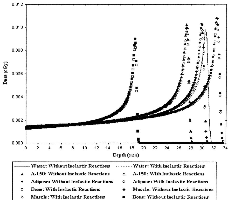
Fig. 3. Comparison of depth-dose distributions for a monoenergetic 60-MeV proton beam in different phantom materials.
