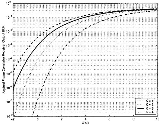
Fig. 5. Barker Code  $K$  interferers,  $E_b/N_o = 20dB$
