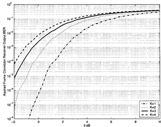
Fig. 6. CCK codes,  $K$  interferers,  $E_b/N_o = 20dB$
