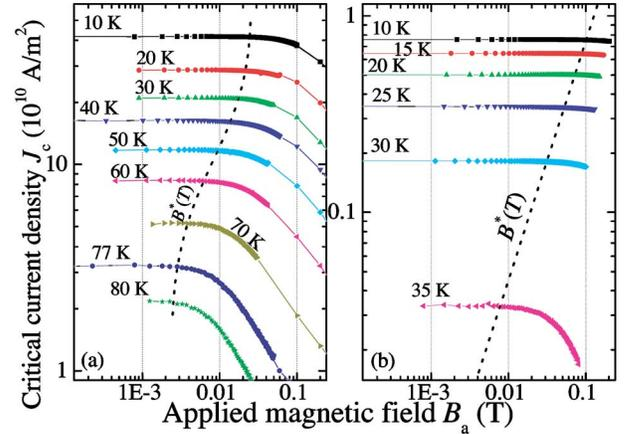
FIG. 1. (Color online)  $J_c(B_a)$  dependences for (a) YBCO (P0311) and (b) MgB<sub>2</sub> (MB2) samples. The dotted lines show  $B^*(T)$ .
