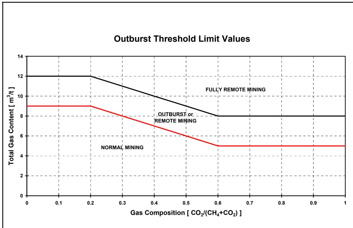
Figure 1 - Typical outburst Threshold Limit Value (TLV) graph
