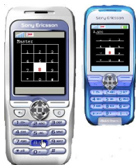
Figure 2 shows a single key ("8") pressed on the master device (larger phone). The corresponding key appears in the MIDlet which displays the pressed key on both the master and the slave devices.
