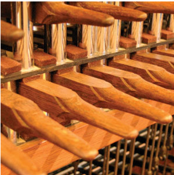
Figure 1. The clavier keys of a carillon. Courtesy of the National Carillon, Canberra, Australia.
