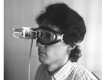
Figure 1. User wearing the eye camera.
