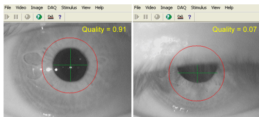
Figure 3. Image analysis of iral signature: high quality (left), low quality (right, blink).
