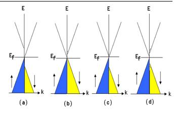
FIG. 4 (color online). Energy band diagrams for spin gapless semiconductors with linear dispersion between energy and momentum.
