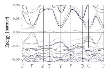
FIG. 7 (color online). Spin-resolved band structure of  $PbPdO_2$ . Majority spin (solid lines) and minority spin (dashed lines).
