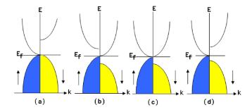
FIG. 3 (color online). Energy band diagrams for spin gapless semiconductors with parabolic dispersion between energy and momentum.
