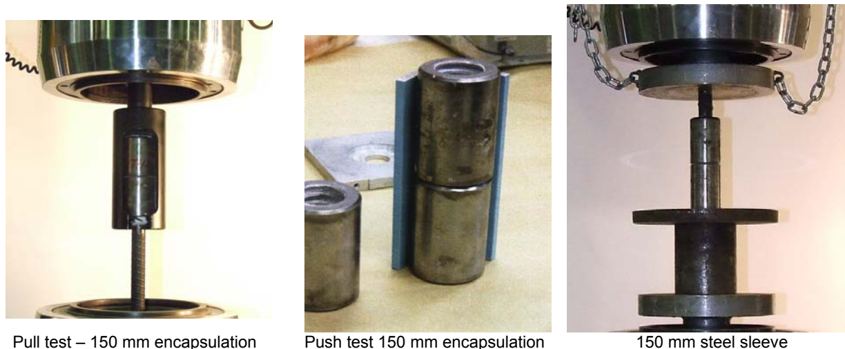
Figure 4 - Pull and push testing of bolts with different encapsulation length of 115 and 150 mm
