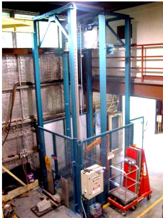
Schematic Figure 7 - Large capacity impact load test facility at UoW
