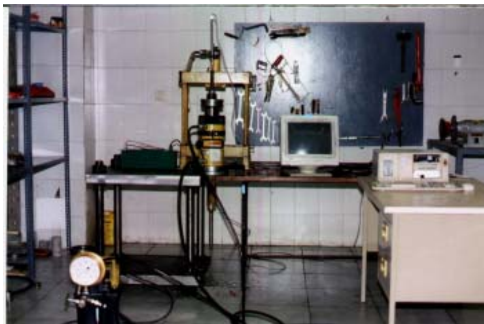
Figure 3 - Test setup with the hollow ram jack and DAS system for data collection.
