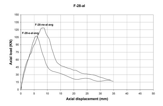
Figure 8 - 28 mm rebar results for epoxy coated (e) and non epoxy coated (ne) when confined in aluminium pipe.
