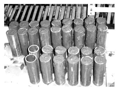
Figure 2 - Grout samples poured for mechanical properties tests.
