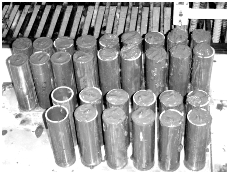
Figure 2 - Grout samples poured for mechanical properties tests.
