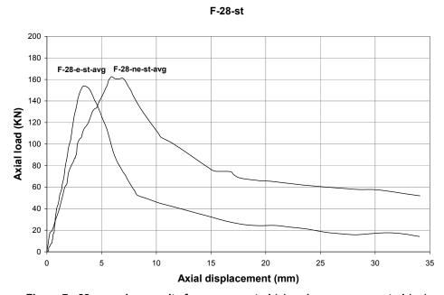
Figure 7 - 28 mm rebar results for epoxy coated (e) and non epoxy coated (ne) when confined in a steel pipe
