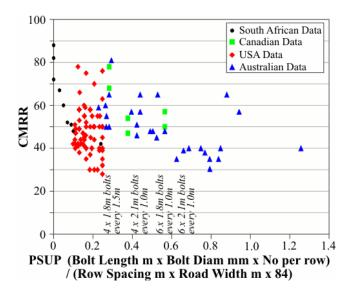
Figure 9 - PSUP (primary support density) versus CMRR.
