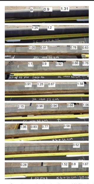
Figure 4 - Core photographs showing diametral PLT Is50 values
