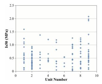
Figure 3 - Diametral pointload test Is50 by unit
