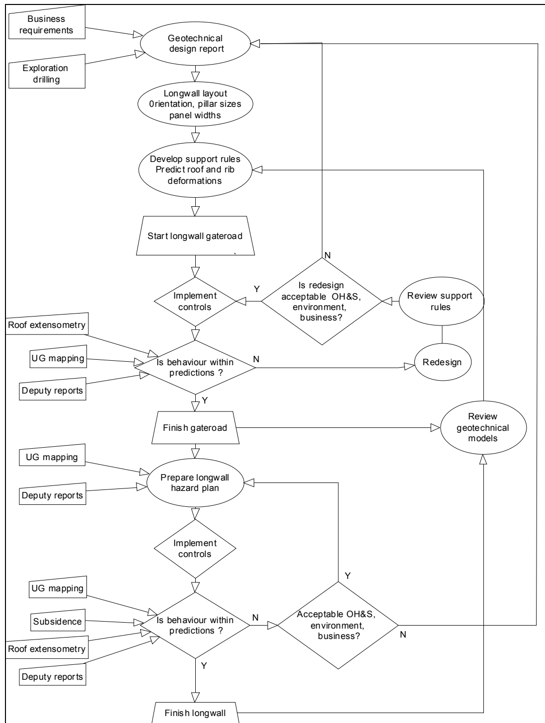
Figure 2 - A model for the integration of geological and geotechnical programs into longwall design, planning, and operations (diamonds – SMT, ovals – geotechnical designer)
