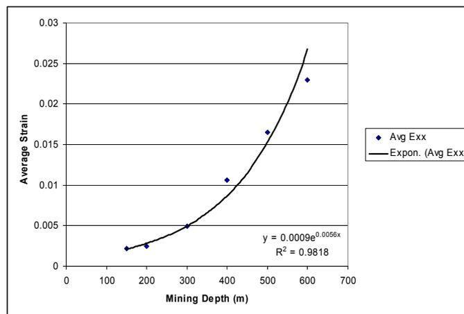
**Figure 9 - Plastic strain verse mining depth**
