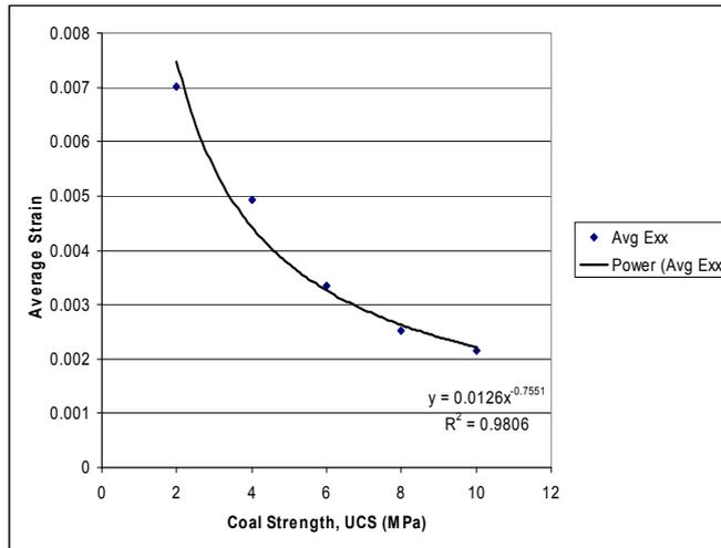
**Figure 8 - Plastic strain verse coal strength**
