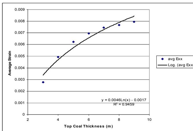
**Figure 10 - Plastic strain verse top coal thickness**
