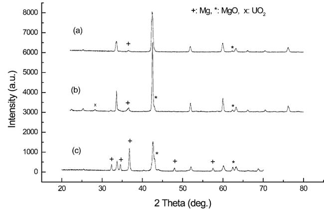
Fig. 1. XRD spectra of the  $\text{MgB}_2$  used for the samples. (a) Undoped, sintered at  $900\ \text{°C}$  for 3 h; (b) doped with 1 wt% U as  $\text{UO}_2$ , sintered at  $900\ \text{°C}$  for 3 h; and (c) undoped, sintered at  $760\ \text{°C}$  for 0.5 h.  $\text{MgB}_2$  phase peaks are unmarked.
